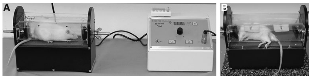
FIG. 1. Setup of the rat Galileo-device for whole-body vibration (WBV) training. During conditioning (A), intact rats received WBV at 15 Hz for 5 min daily. WBV therapy (B) started at 7 or 14 days after SCI and consisted of five sequential trials of vibrations at 15 Hz and 30 Hz (see text for more details).
