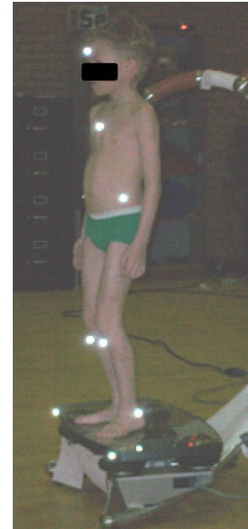
Fig. 1. Vibration platform set-up and typical posture chosen by participants. Reflective markers highlight location of skeletal landmarks.
